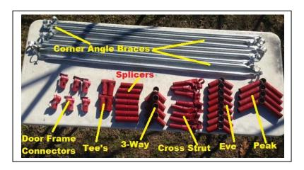
This kit requires 16 gage or heavier 1 3/8" chain link fence top rail tubing. Here we are building a 12'x12' greenhouse frame however you can change the width and frame spacing to meet your own needs.
